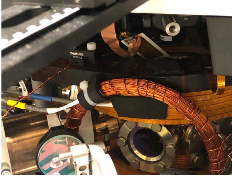
Figure 2.6: The N = 2 microwave antenna mounted above the science chamber. The antenna is positioned at an angle to avoid obstructing the optical access for the ODT and ionization beams from above.
